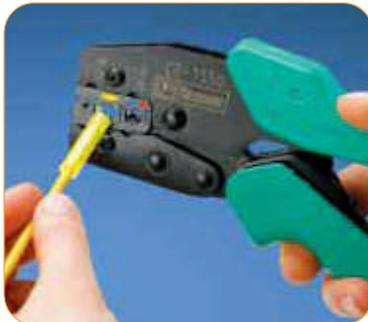
Suitable for in-line, parallel and group splicing of wires
